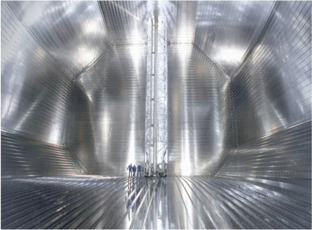
Membrane no 96 Gas Transport en invar
